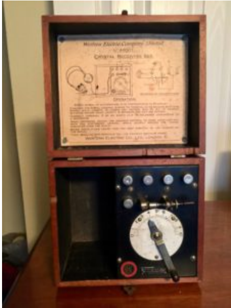
WESTERN ELECTRIC MODEL 44001 CRYSTAL RADIO
