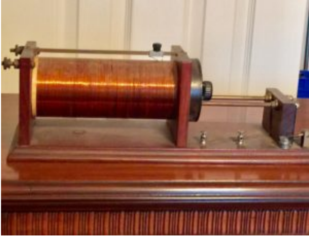
Homebrew loose coupler crystal radio
